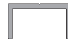
AYPC.SF.3603 Channel spacer for concealed door closer slide channel installation matching with AYPC.SF.3202, AYPC.SF.3204, AYPC.SF.3205
